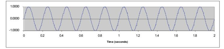
Mathematically this is a 'sin' curve. Signal intensity at time t is  $sin(2\pi ft)$ , where f is the signal frequency measured in cycles per second. In the graph above there are 10 cycles (10 peaks and 10 troughs) in 2 seconds, giving a frequency of 5 cycles per second.
