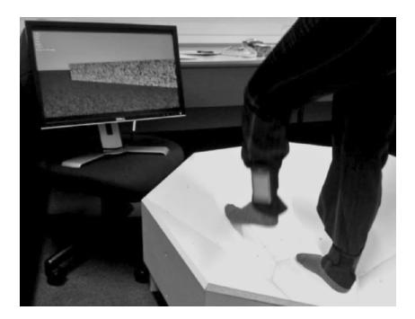
The cellphones record accelerometer data approximately 100 times per second. You have been supplied with a record of a little over 14 seconds of data from Rachel's right leg. Each row of your data holds one observation with four numbers. The first is the time in
